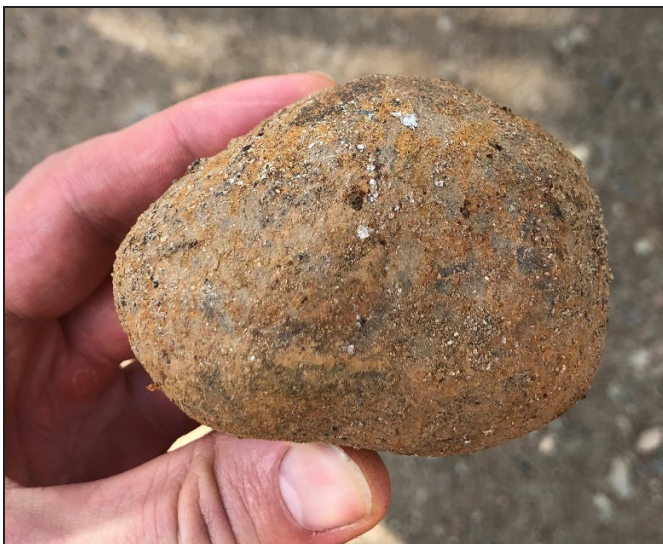
Figure 14. Deformed grinding media
