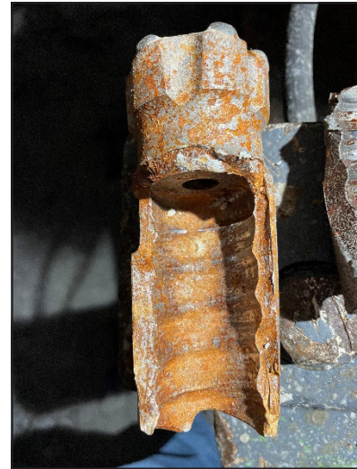
Figure 9. Broken thread, resulting from insufficient torque and/or excessive side loading
