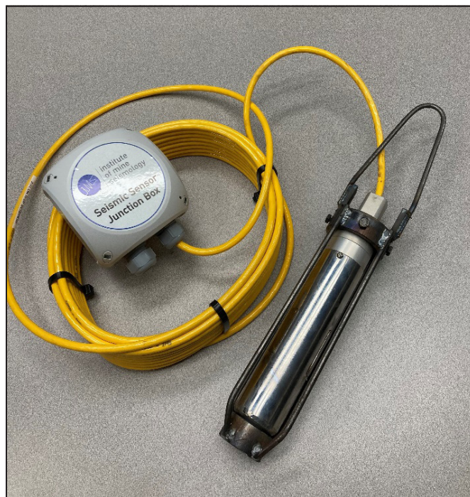
Figure 9. IMS Model 3G14 geophone (after Institute of Mine Seismology, 2013)
