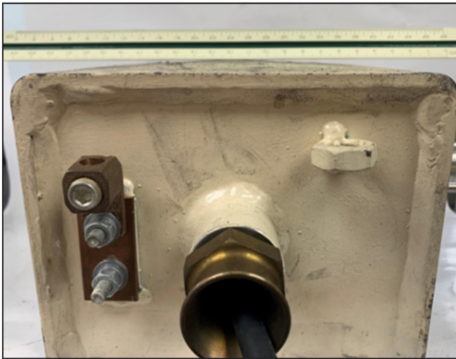
Figure 12. Thermal runaway pressure deformed the XP enclosure bottom plate beyond allowable limits
