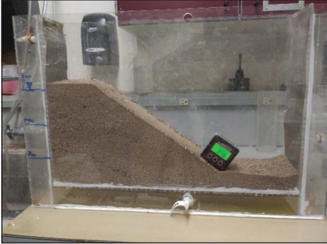
Figure 6. Box of soil sample before gradual water rise experiment
