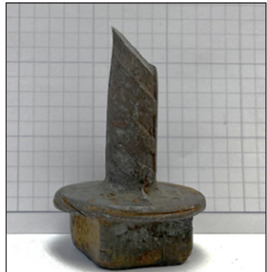
Figure 8. Head portion of fractured bolt showing necking behavior induced by FGPT
