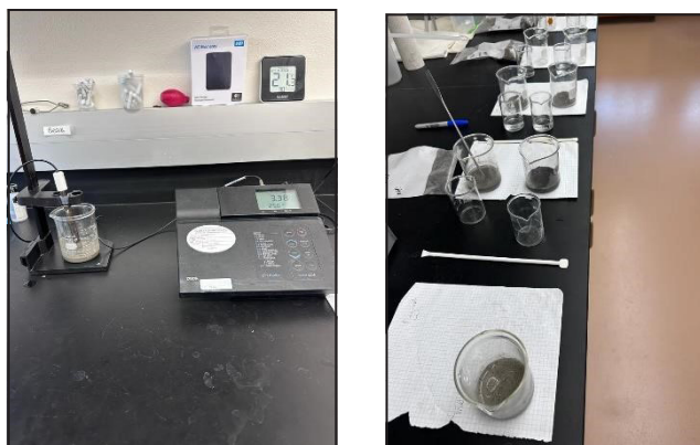
Figure 5. Paste pH test on sieved samples
