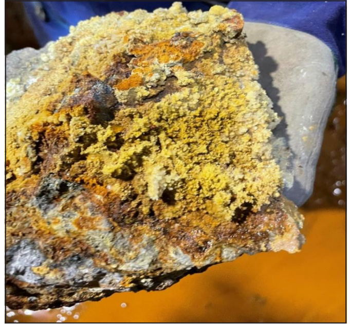
Figure 5: Examples of corrosion precipitates from TPL2(68L) indicates hydroxysulfates such as jarosite [ \text{KFe}(\text{SO})(\text{OH}) ]. From Logston, 2022
