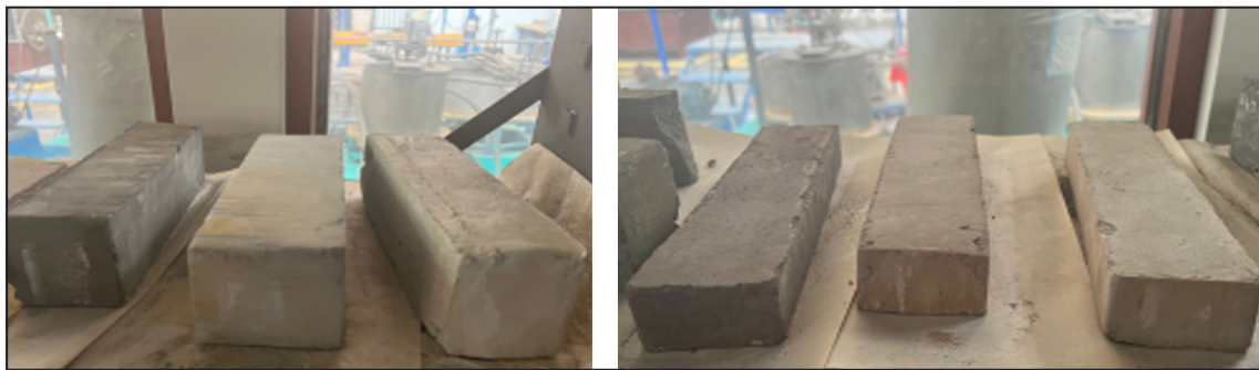
Figure 3. Manufactured bricks using final tailings from flotation tests
