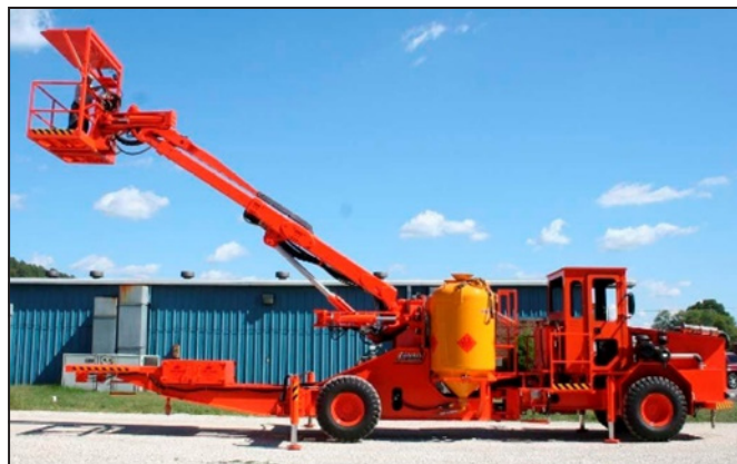
Figure 2. ANFO loader with basket (the DCAC would be inserted over the basket)
