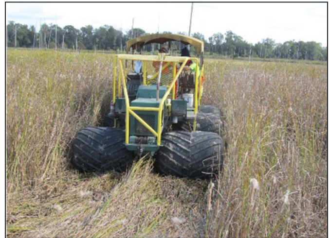
Figure 6. Amphibious CPT rig (courtesy R. B. Jergens)
