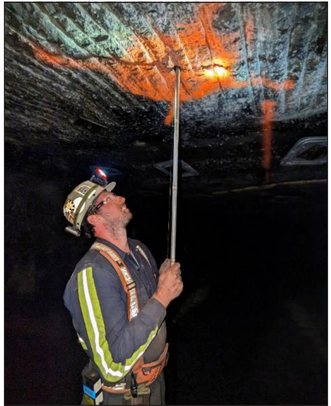
Figure 9. Photo of a researcher beginning the process of installing anchors for a roof extensometer
