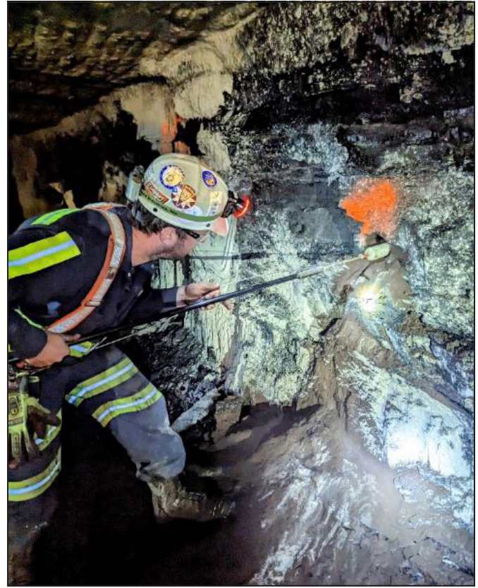
Figure 7. Photo depicting a researcher beginning the installation of a BPC using a set of insertion/setting rods
