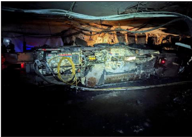
Figure 2. Example of tramming a continuous miner representing a potential struck-by hazard
