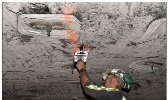
Figure 10. Photo of a researcher completing the installation of a roof extensometer using epoxy and wooden wedges.
