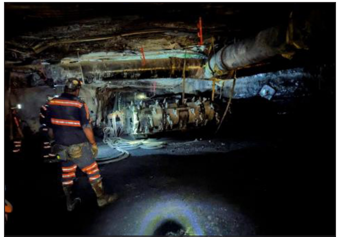
Figure 3. Example of a tramming continuous miner depicting the tight spaces associated with underground equipment and potential for caught between hazards
