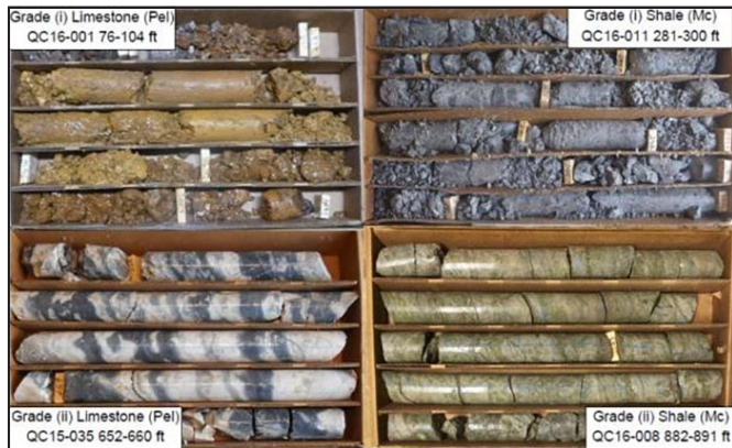
Figure 1. Visual comparison of the different alteration grades on core samples (Yong, et al, 2022).
