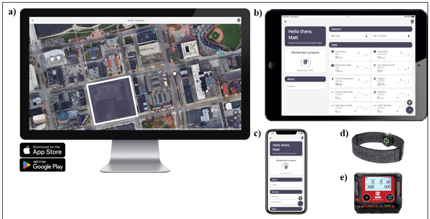
Figure 2. Images representing the technologies used within the trial. a) SafeGuard Live web view, b) SafeGuard Live, tablet view, SafeGuard Live, phone view, d) Polar Verity Sense heart rate monitor with armband, and e) RKI GX-3R Pro multi-gas chemical sensor
