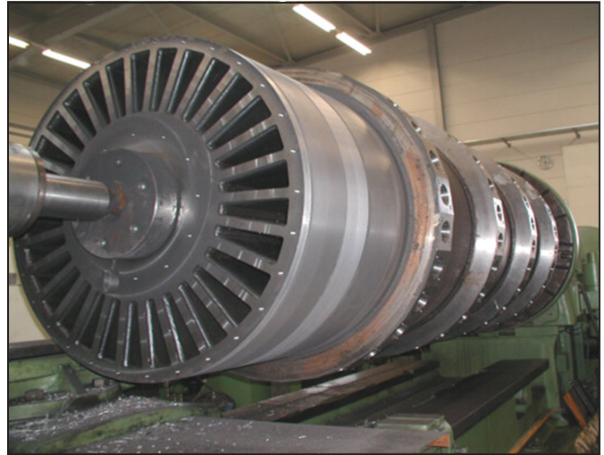
Figure 10. View of new filter barrel with stainless steel filtrate pipes
