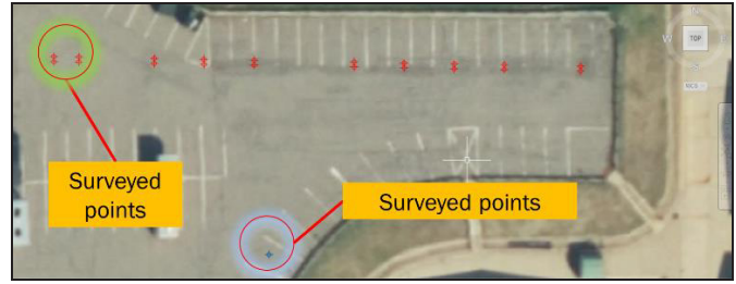
Figure 1. Test setup for static and dynamic tests. Starting from the top left, the two rows of points represent the ground truth marked by the RTS and the point on the bottom is the point surveyed for the base station
