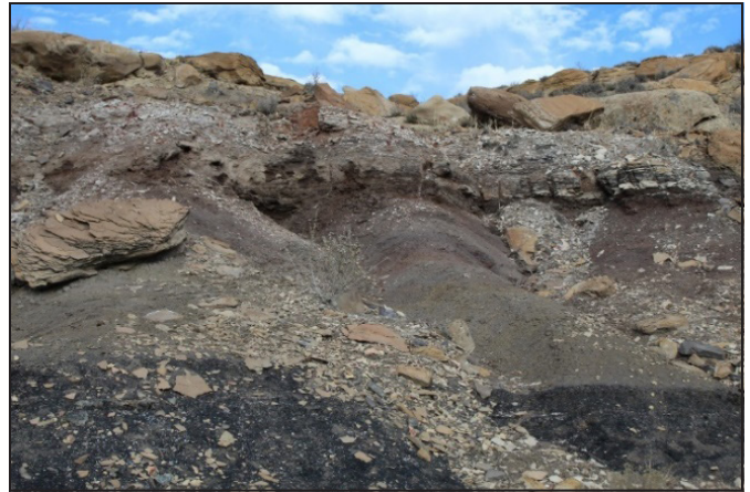
Figure 3. Humate mine in the Star Lake field, northern New Mexico. The humate is the upper brownish layers overlying the black coal
