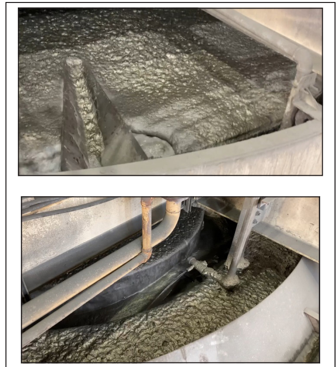
Figure 2. Photo comparison between both launder configurations, radial launders (left) and center launder (right) in Kennecott (2022)
