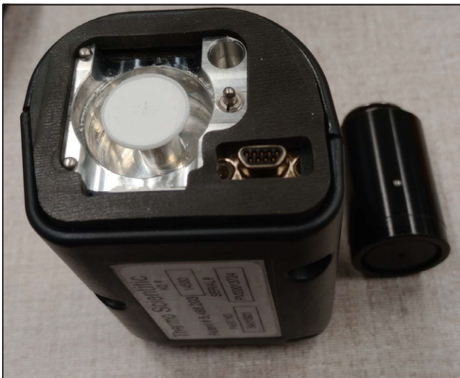
Figure 5. The new PVC filter for silica analysis shown attached to the CPDM transducer where the respirable dust sample is collected
