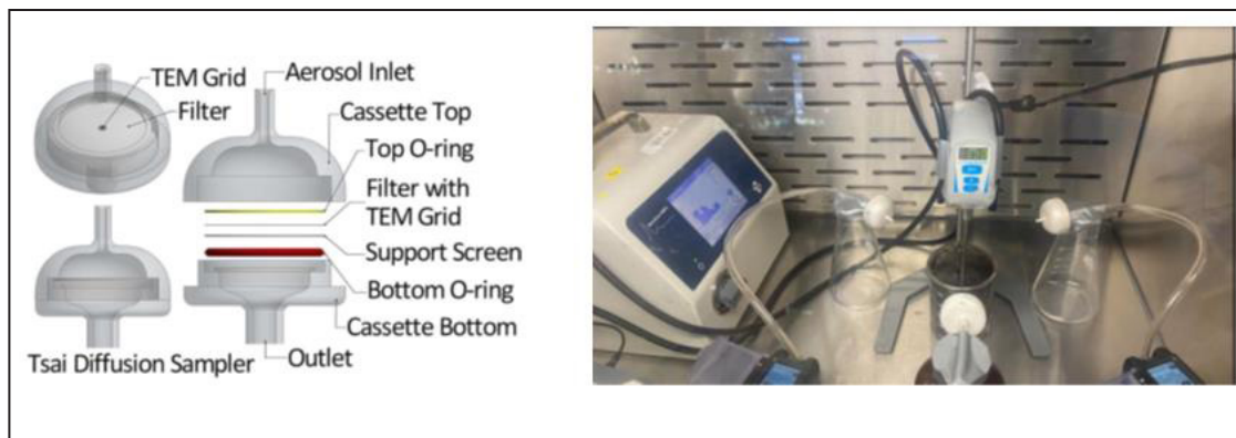
Figure 1. The Tsai diffusion sampler components (left) and the experimental test setup used to test the Tsai diffusion sampler (right)
