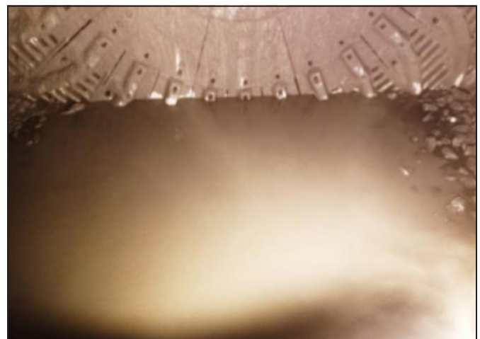
Figure 9. SAG mill slurry pooling
