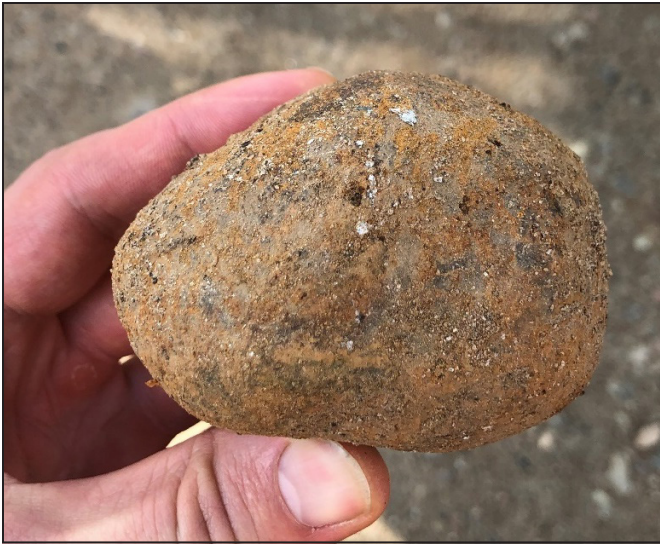
Figure 14. Deformed grinding media
