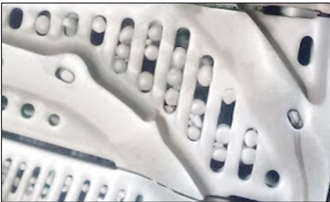
Figure 15. Deformed grinding media blinding SAG mill discharge grates
