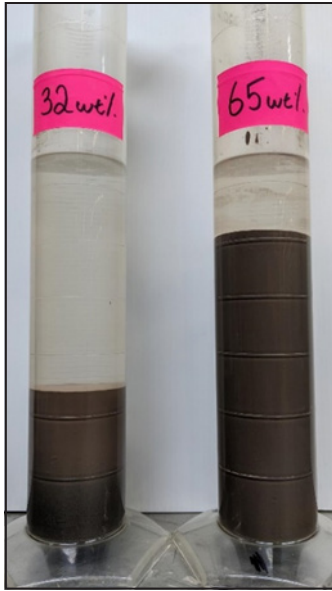
Figure 3. The effect of improved dewatering. Left the current slurry at 32% solids concentration by weight, on the right the slurry at 65% solids concentration by weight
