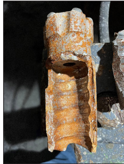
Figure 9. Broken thread, resulting from insufficient torque and/or excessive side loading
