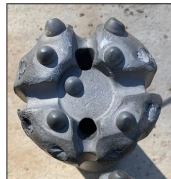
Figure 10. Premature button breakage, resulting from too slow rotation and/or broken ground
