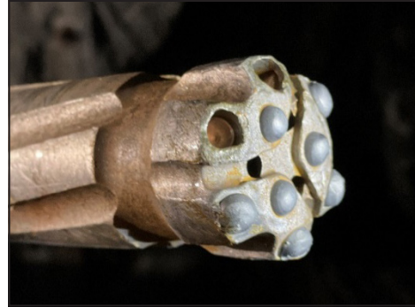
Figure 8. Lost buttons, resulting from poor collaring using too much power and/or no rotation
