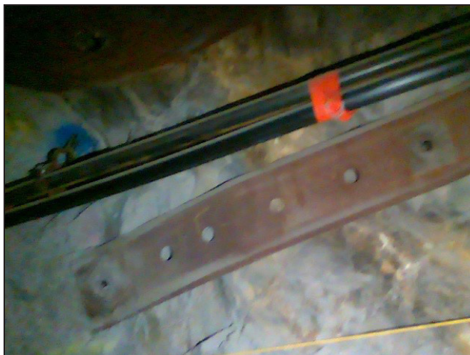
Figure 3. Shows an image of the roof from a typical point-of-view of a roof bolting drill. It is critical to be able to differentiate the strap from the rock
