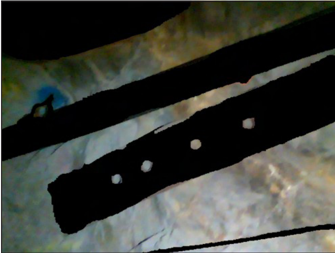
Figure 6. Shows the result of the alpha matting algorithm where the boundary between the rock and strap has been drawn. This mask can be processed to eventually be ground truth
