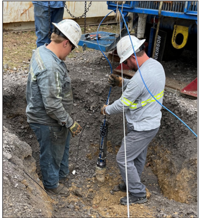
Figure 10. Photo depicting the initial installation of an IMS Model 3G14 geophone into a gas well
