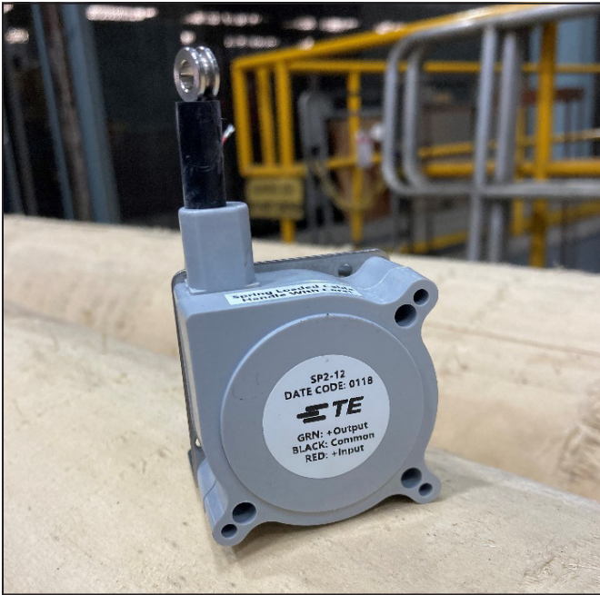
Figure 2. Example of a string potentiometer
