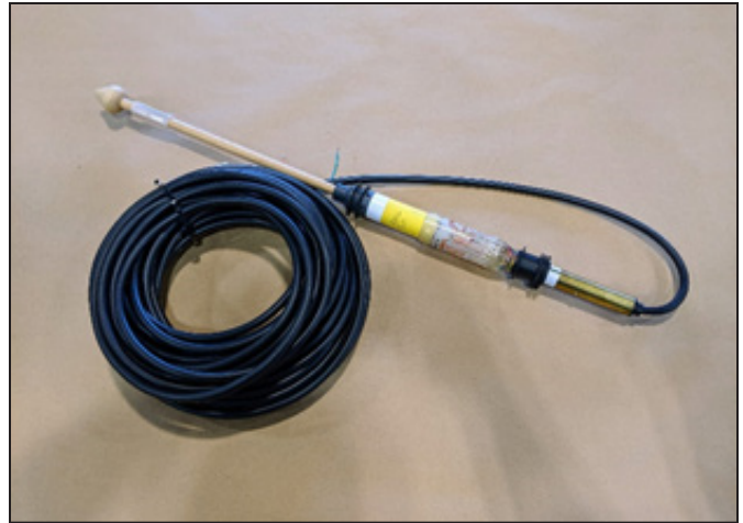
Figure 13. Hollow Inclusion (HI) Cell depicting the cell itself, plunger, wooden dowel, and a pre-selected length of cable
