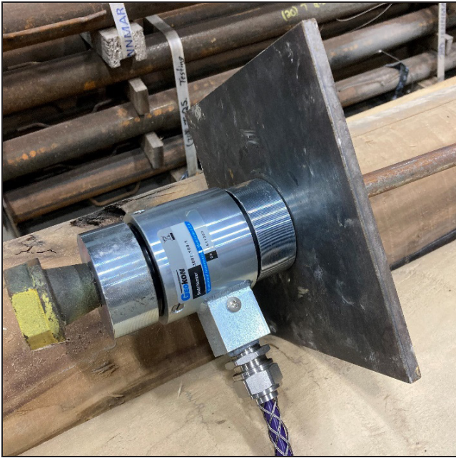
Figure 15. Example of a GEOKON Model 3000 load cell (after GEOKON, 2020)
