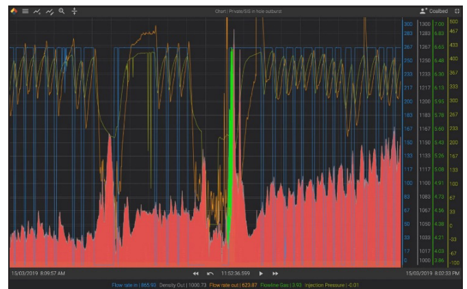
Figure 5. Outburst event measured downhole. Note sudden peak gas influx (green) and steadily increasing density of returning drilling fluid (red) due to structure-related crushed coal flowing into the borehole
