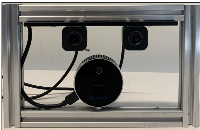
Figure 5. Cameras Setup for Collecting Real Data. Two Event Cameras and L515 LiDAR Camera.
