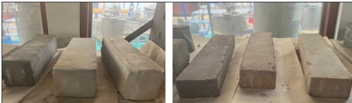
Figure 3. Manufactured bricks using final tailings from flotation tests
