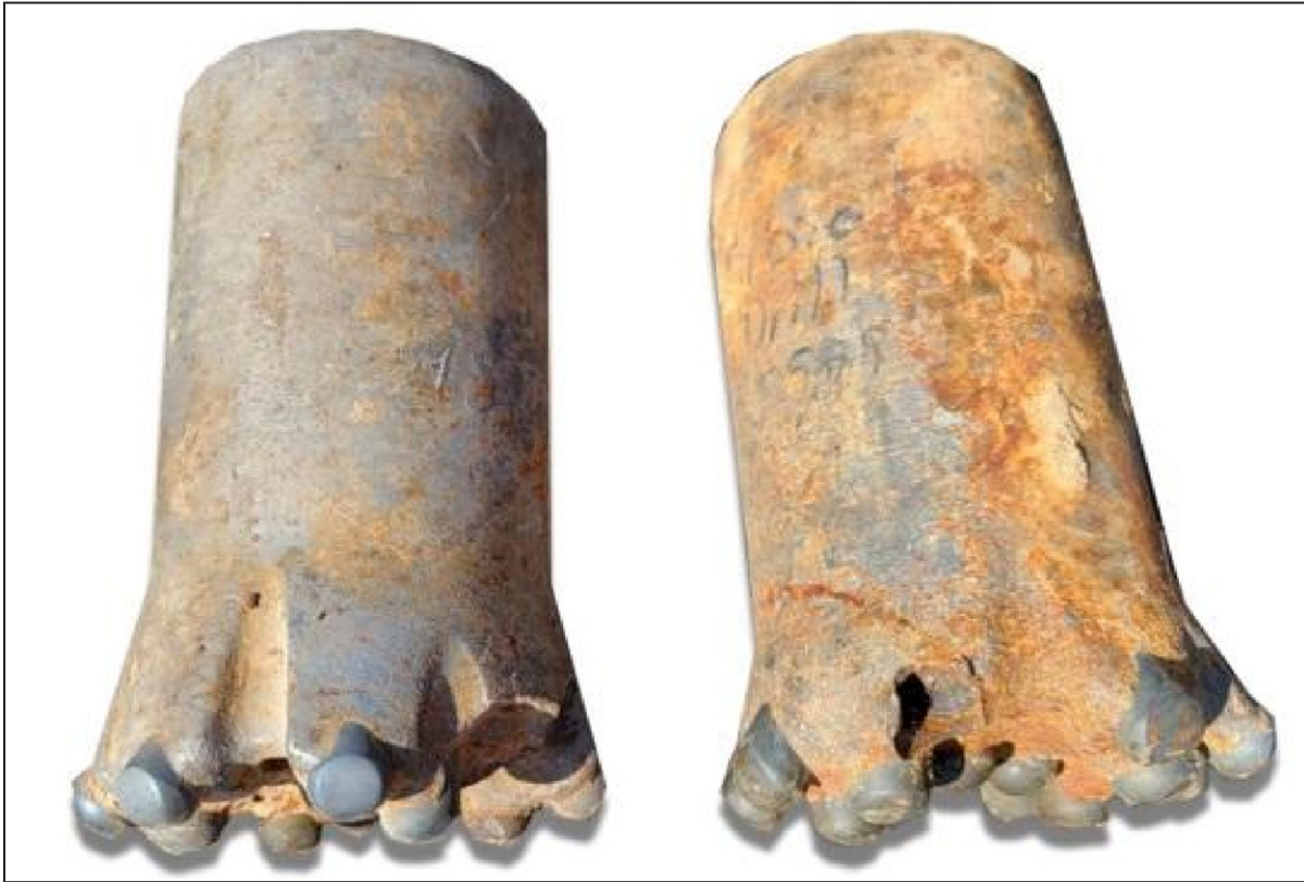
Figure 1. Untreated bit with failure at 4,907 ft (left). The treated bit with 12,999 ft (right) from the same manufacturer
