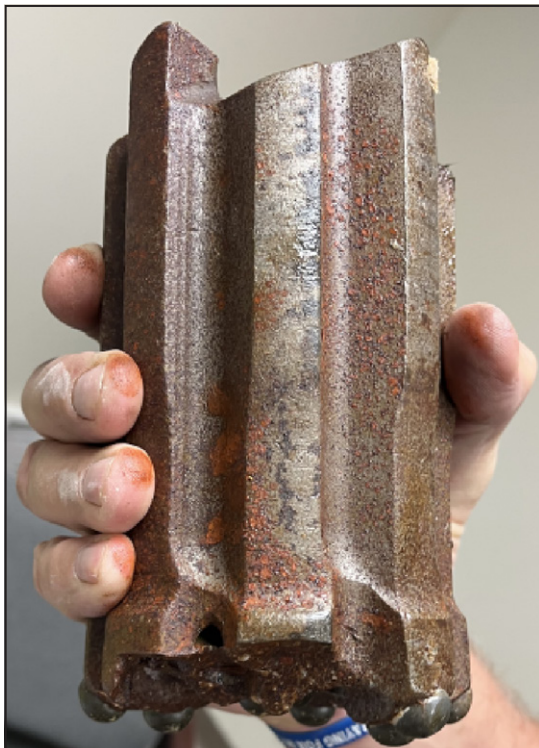
Figure 2. Side view of Treated Bit 1 with breakage failure
