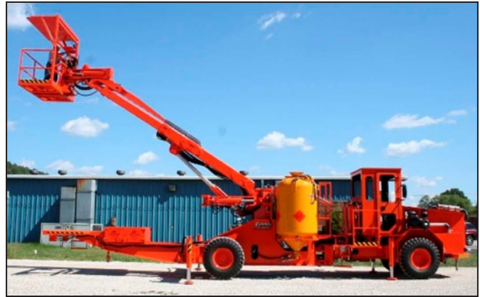
Figure 2. ANFO loader with basket (the DCAC would be inserted over the basket)
