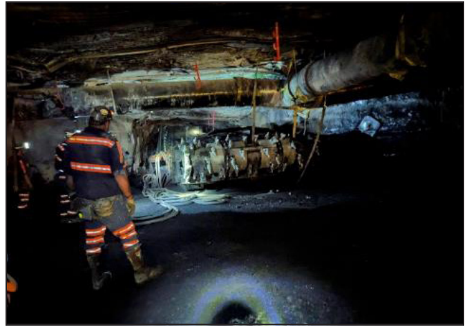
Figure 3. Example of a tramping continuous miner depicting the tight spaces associated with underground equipment and potential for caught between hazards
