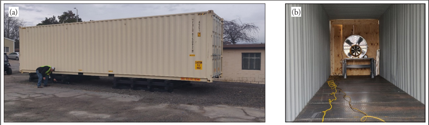
Figure 1. Steel shipping container (a) outside and (b) inside, modified to be used as a fire suppression test facility
