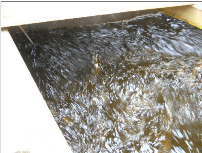
Figure 4. Typical turbulent solution surface in the E1B mix box with R301 impeller
