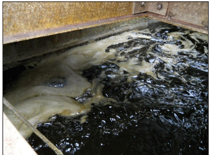
Figure 5. Typical semi-quiescent solution surface in the E2B mix box with R320A impeller
