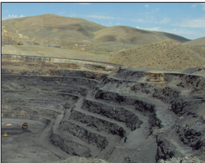
Figure 7. A July 2010, photograph that shows the upper benches of the highwall above the proposed portal location
