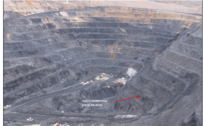
Figure 8. This January 2011 photograph shows the highwall above the proposed portal location. Development of the existing portals has commenced in the northern end of the pit.
