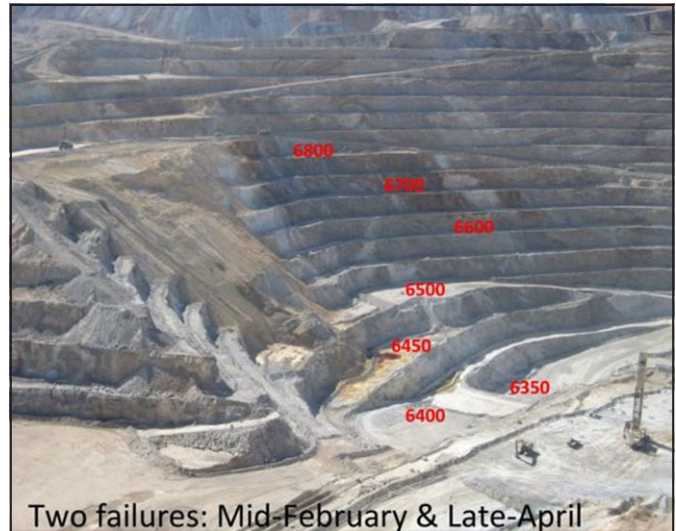
Figure 4. Photograph showing the high-wall movement on the eastern side of the pit (Yang, 2015).
